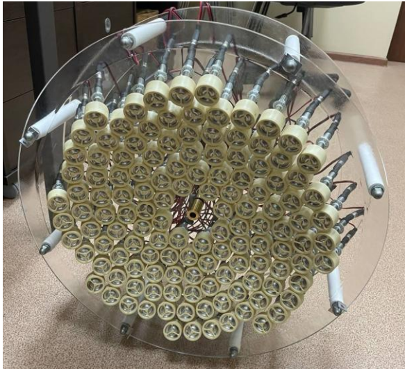
Figure 1. Photo of 128-element focused ultrasound array used in the current study
