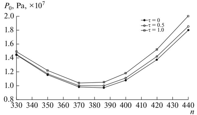
**Fig. 3.** First zone of instability of a drop surface in parameters  $(P_0, n)$  at different moments of slow time.
