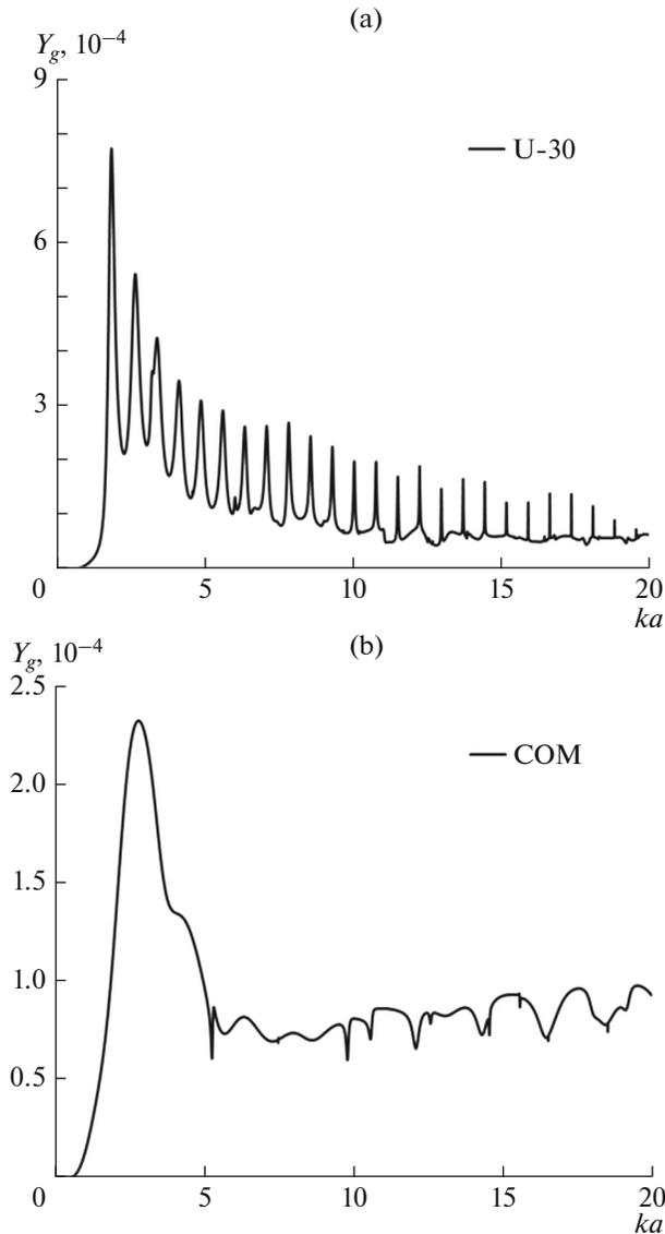
**Fig. 1.** Dependence of normalized values of the radiation force on parameter  $ka$  at a fixed ratio of the beam radius to the scatterer radius ( $a_0/a = 1$ ) for two types of materials: (a) U-30 and (b) COM.
