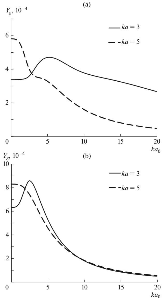
**Fig. 2.** Dependence of the normalized values of the radiation force on the waist radius of a quasi-Gaussian beam at different fixed values of parameters  $ka$  ( $ka = 3, 5$ ;  $a = 2.5$  mm). The diagrams are plotted for two types of elastic spherical scatterers: (a) U-30 and (b) COM.
