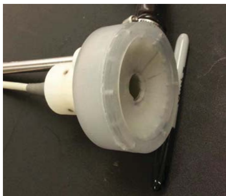
Figure 1: 12-element 1.5 MHz HIFU sector array transducer integrated with an ultrasound imaging probe (ATL P7-4).
