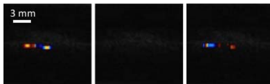
FIGURE 3. Results of the overpressure experiment on natural kidney stones. From the left to the right: twinkling is seen before increasing pressure (left), no twinkling is present during the high-pressure of 8.5 MPa (middle), and twinkling returns after the pressure is released (right).
