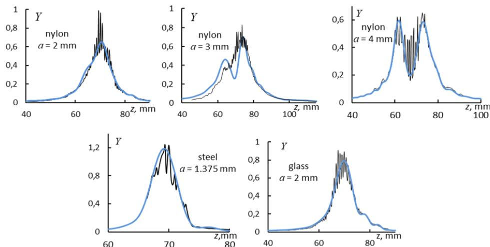
Figure 3: Numerical curves (blue) and experimental results (black) from measuring the radiation force for the scatterers.
