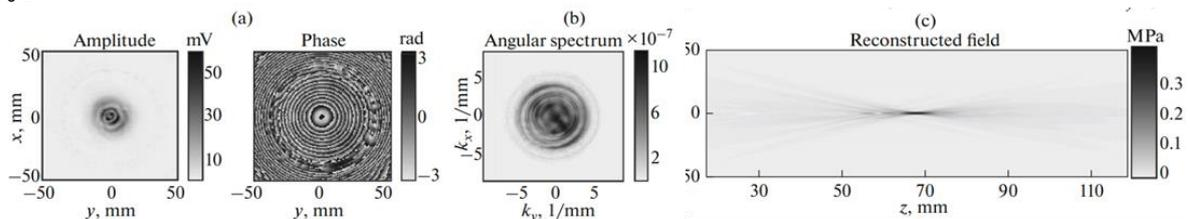
Figure 1: (a) Measured field amplitude and phase in the transverse plane of a transducer at  $120 \times 120$  points with a spacing of 0.5 mm; (b) reconstructed angular spectrum of the transducer; (c) pressure field of the focused beam in the plane.
