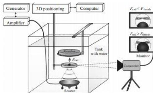
Figure 2: Experimental set-up for measuring the radiation force acting on elastic spherical scatterers.
