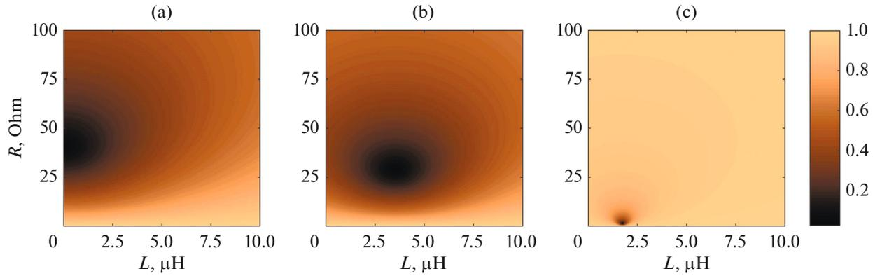
**Fig. 2.** Absolute value of the reflection coefficient as a function of inductance and resistance connected in parallel to the piezotransducer operating in the transmit mode at different frequencies of incident acoustic waves: (a) 1.117, (b) 1.13, and (c) 1.2 MHz.
