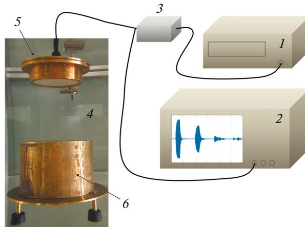
**Fig. 3.** Scheme of the experimental setup: (1) generator, (2) oscilloscope, (3) active resistance of 1 kOhm, (4) water tank, (5) piezoelectric transducer, and (6) brass cylinder used as a reflector.
