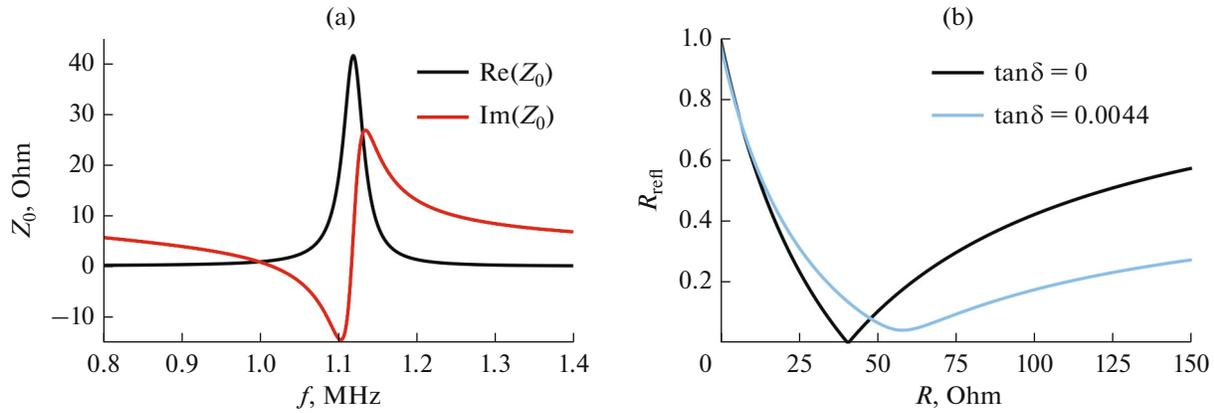
**Fig. 1.** (a) Real and imaginary parts of the impedance of the piezotransducer; (b) absolute value of the coefficient of reflection of an incident plane acoustic wave off the piezoplate, as a function of the active load at the frequency of antiresonance using two values of the piezoceramic's loss factor.
