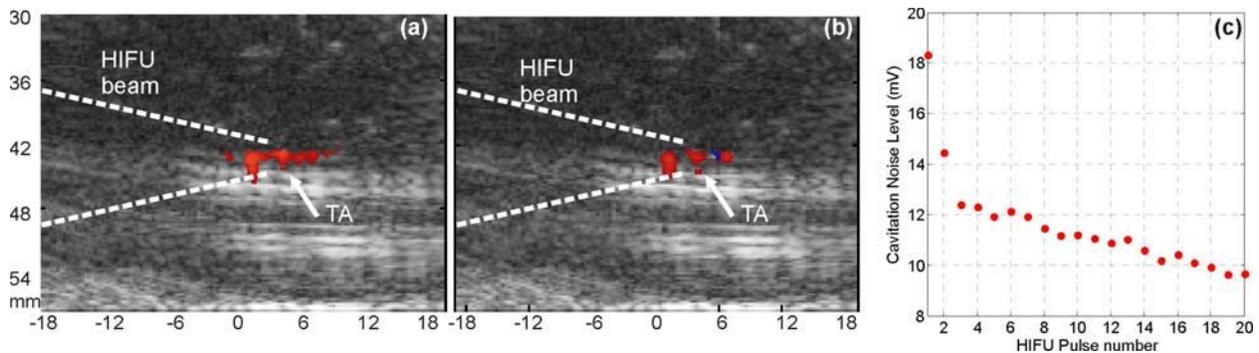
**FIGURE 2.** Ultrasound images (Doppler and B-mode) acquired during a single 20-pulse HIFU exposure of a polyacrylamide gel phantom after the 1<sup>st</sup> HIFU pulse (a) and after the 11<sup>th</sup> HIFU pulse (b). Cavitation noise level detected by the PCD during the exposure (c). Over the course of the exposure, the cavitation activity declined, and so did the brightness and the size of the TA. Note, that the brightness of the B-mode image did not change.
