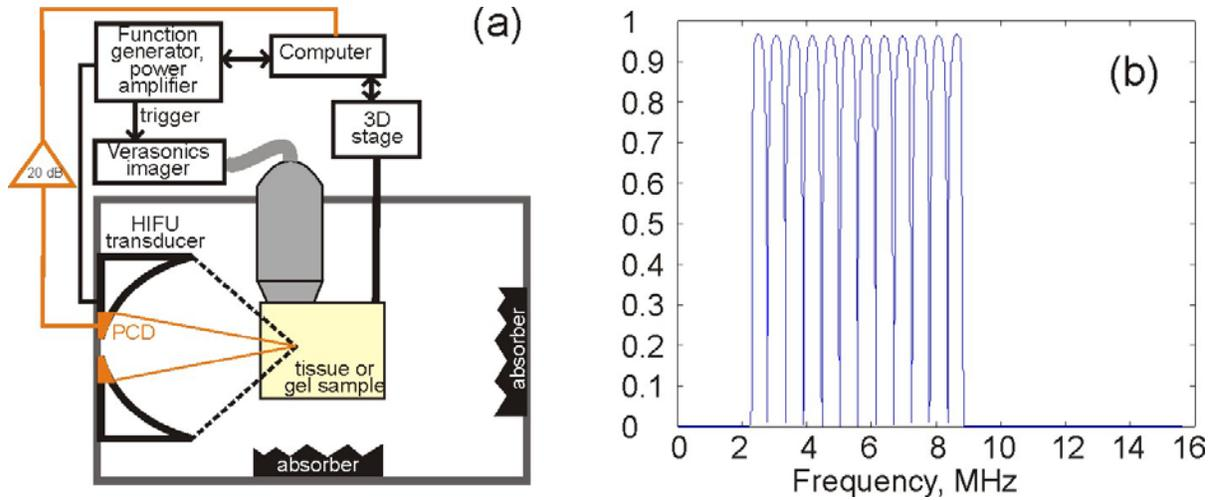
**FIGURE 1.** (a) Schematic illustration of the experimental setup. (b) The combination of the band-pass and notch filters applied to the PCD signals in the frequency domain.
