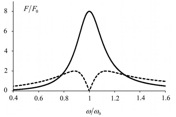
FIG. 13. Plot of magnitude of the normalized radiation force  $F/F_0$  on a bubble with  $Q = 4$  versus normalized frequency  $\omega/\omega_0$  in a standing or traveling wave:  $F_{\text{traveling}}/F_0$  is shown with a solid line and  $F_{\text{standing}}/F_0$  is shown with a dashed line. The standing wave has a null exactly at resonance, but far from resonance, the force is larger than for traveling waves.
