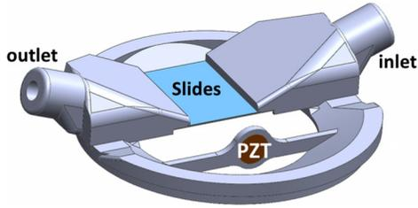
FIG. 5. (Color online) Microscope coverslips were sandwiched together, separated by 87- $\mu\text{m}$  wires attached at the corners. The slips were mounted to a 3-D printed fixture so that a suspension of cells could flow between them. A PZT transducer operating at 1 MHz generated pulses of ultrasound that displaced cell-MB conjugates. The entire housing was submerged in degassed water and aligned under a microscope for imaging.
