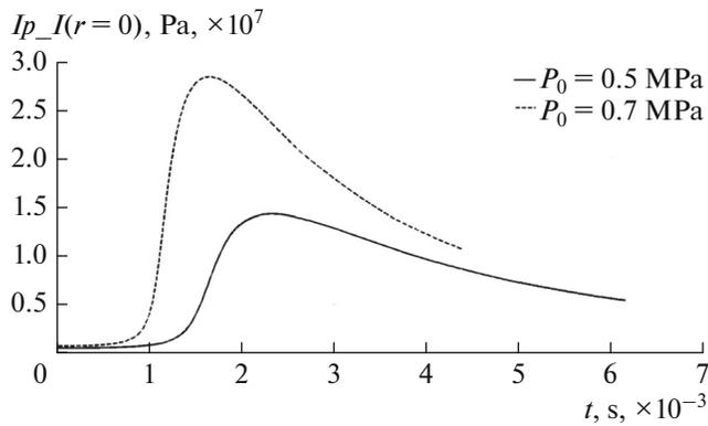
Fig. 1. Peak pressure in the center of a drop.
