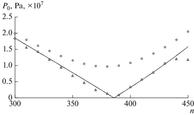
**Fig. 2.** First zone of instability of a drop surface in parameters  $P_0$  (the pressure at the center of the drop at the initial moment):  $n$  is a harmonic number; the black line is for theoretical calculations without viscosity;  $\Delta$  represents numerical calculations without viscosity;  $\circ$  denotes a numerical calculations with viscosity.
