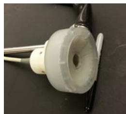
Figure 1. Focused ultrasound transducer of 1.5 MHz frequency used in the study.
