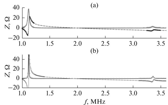
**Fig. 5.** Comparison of imaginary and real parts of impedance experimentally measured (squares and circles, respectively) and theoretically calculated (gray and black solid lines, respectively) for measurements in (a) water and (b) air in wide frequency range.
