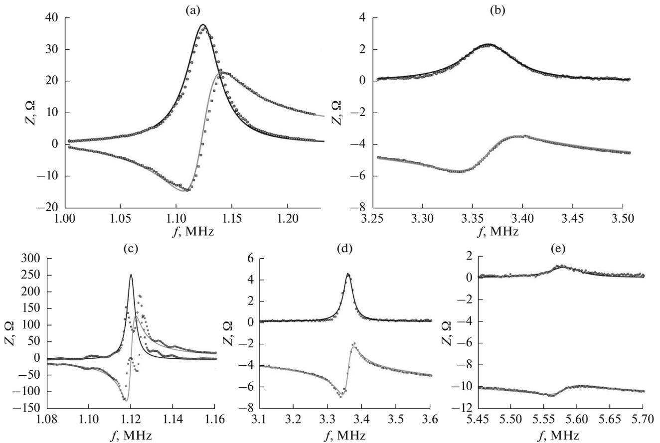
**Fig. 4.** Comparison of imaginary and real parts of impedance experimentally measured (squares and circles, respectively) and theoretically calculated (gray and black solid lines, respectively) for measurements (a, b) in water and (c–e) in air at resonance frequencies.
