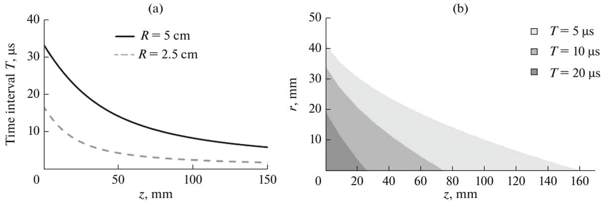
**Fig. 1.** (a) Estimate of time interval during which plane wave pulse is realized on axis of symmetry of transducers with radii of 5 and 2.5 cm as function of distance to center of transducer; (b) estimate of dimensions of plane wave region in directions along and across beam axis for plane wave intervals of 20, 10, and 5 μs.
