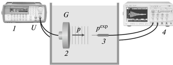
**Fig. 6.** Diagram of experiment on emission and reception of plane wave. 1, generator; 2, piezoelectric transducer; 3, hydrophone; 4, oscilloscope.
