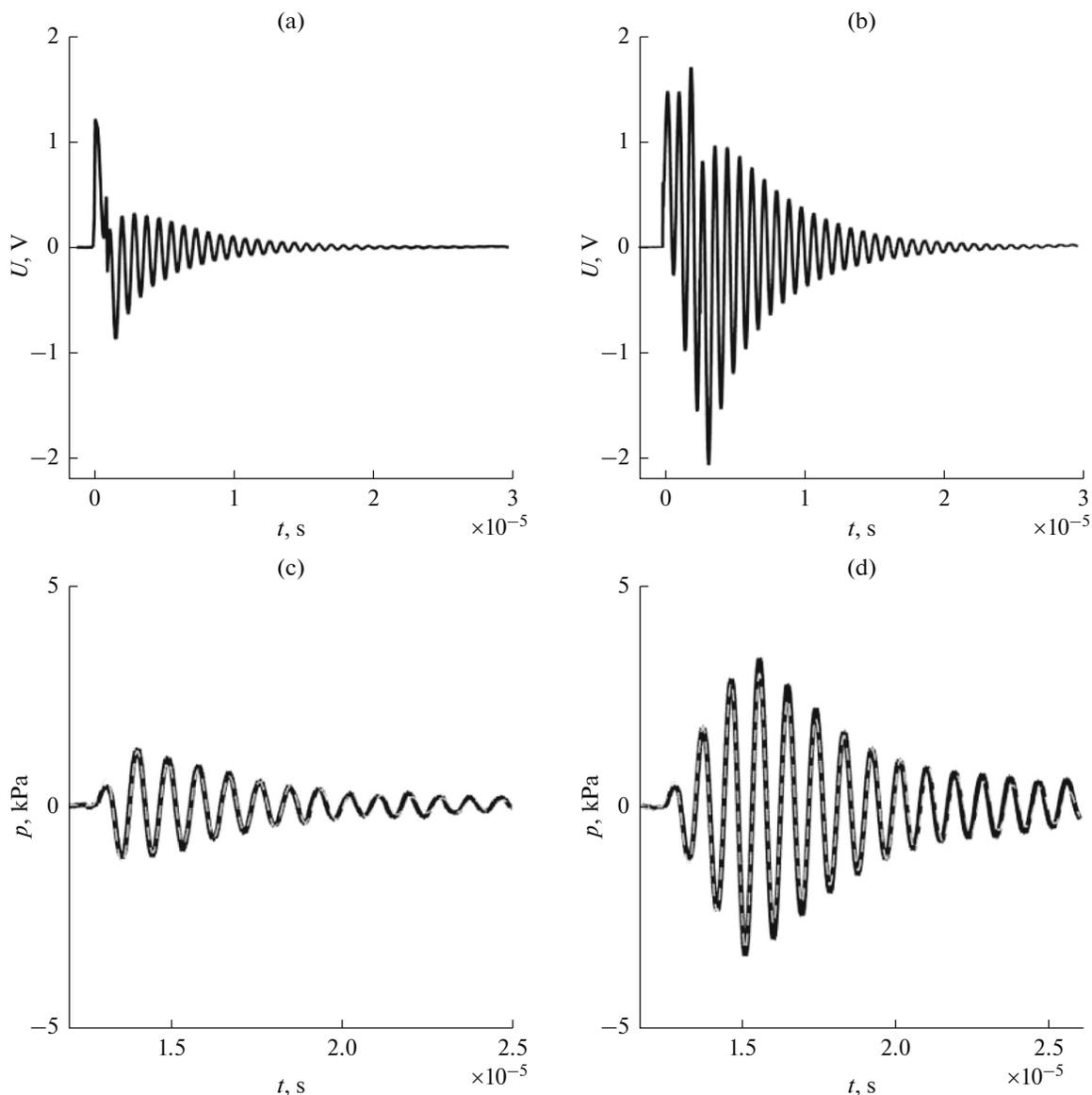
**Fig. 7.** Electrical signal measured at the transducer with the shape of the electrical signal at the generator in the form of (a) one sine period at resonance frequency and (b) three sine periods at resonance frequency; (c, d) comparison of corresponding experimentally measured pressure signal (black line) with theoretically calculated one (gray line).
