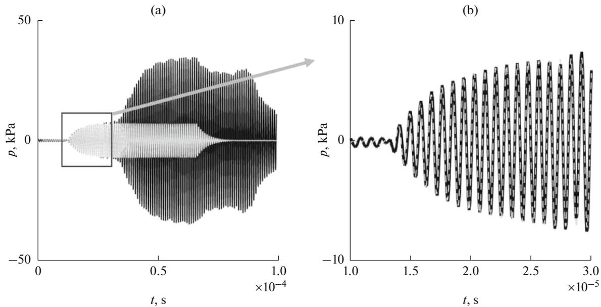
**Fig. 8.** Comparison of experimentally measured signal (black line) with theoretically calculated one (gray line) for quasi-harmonic electrical signal (60 sine periods at resonance frequency set on generator).
