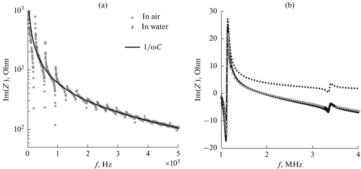
**Fig. 3.** (a) Approximation of imaginary part of experimentally measured impedance by hyperbolic dependence in low-frequency region to determine capacitance of clamped transducer, (b) comparison of experimentally measured frequency dependence of imaginary part of transducer impedance (circles) with theoretical formula for  $Z_0$  disregarding influence of electric cable (dashed line) and dependence for  $Z$  taking into account cable (solid line).
