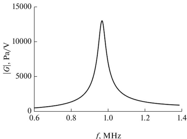
**Fig. 9.** Ratio of pressure emitted by transducer to voltage on transducer as function of signal frequency.
