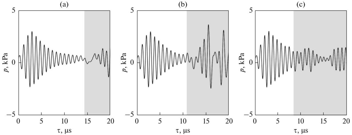
**Fig. 2.** Sweep of signals in coordinates of traveling wave  $\tau = t - z/c_2$  recorded by hydrophone on emitter axis at distances of (a) 10, (b) 50, and (c) 100 mm. Gray color indicates region of recording of edge wave.
